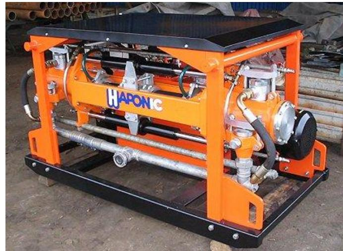
**THE HAPONIC VP 125/400** pump is designed to transport concrete or similar materials.
